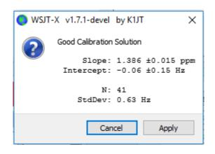
For a quick visual check of the resulting calibration, stay in **FreqCal** mode with the **Measure** option cleared. *WSJT-X* shows the adjusted results directly on the waterfall and the displayed records.
