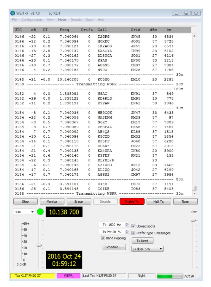
the decodes at UTC 0152, 0154, and 0156 along with the corresponding minutes from the waterfall display below. Yellow ovals have been added to highlight two isolated signals decoded at -28 and -29 dB in the first and third two-minute interval. At 0154 UTC signals from VE3FAL, AB4QS, and K5CZD fall within a 5 Hz interval near audio frequency 1492 Hz; similarly, K3FEF, DL2XL/P, and LZ1UBO fall within a 6 Hz interval near 1543 Hz. Each of the overlapping signals is decoded flawlessly.
