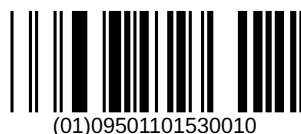
Figure 72: zint -b DBAR_OMN --complantheight -d "0950110153001"
