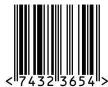
Figure 47: zint -b EANX_CHK --complantheight -d "74323654" --guardwhitespace
