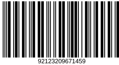
Figure 36: zint -b ITF14 --box --compliantheight -d "9212320967145"
