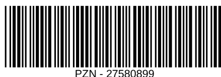
Figure 57: zint -b PZN --compliantheight -d "2758089"
