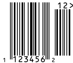
Figure 43: zint -b UPCE --compliantheight -d "1123456+12" --guardwhitespace
