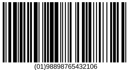
Figure 67: zint -b EAN14 --compliantheight -d "98898765432106"
