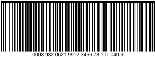
Figure 70: zint -b DPD --compliantheight -d "000393206219912345678101040"
