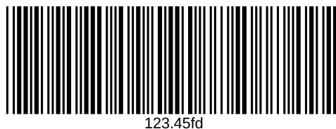
Figure 55: zint -b EXCODE39 --compliantheight -d "123.45$@fd"
