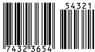
Figure 46: zint -b EANX --complantheight -d "7432365+54321"
