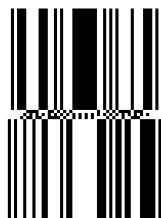
Figure 87: zint -b DBAR_OMNSTK --complantheight -d "9889876543210"
