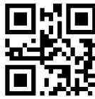
Figure 109: zint -b QRCODE -d "QR Code Symbol" --mask=5
