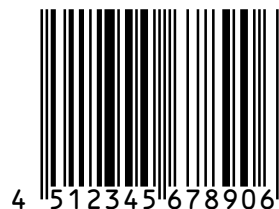
Figure 44: zint -b EANX --compliantheight -d "4512345678906"
