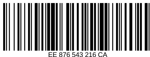
Figure 71: zint -b UPU_S10 --complantheight -d "EE876543216CA"
